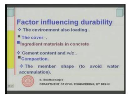
So, so far then we have seen the surface concrete effects. That is 1 thing we have seen, but we have seen more importantly the porosity, pore interconnectivity and pore properties control the concrete durability and this can be controlled through water cement ratio and also through somewhat through cement minimum cement content.
