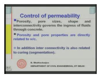
As the age increases proficient of permeability reduces down, because hydration takes place and capillary pores are reduced with hydration capillary pores are reduced. Remember the equation for capillary porosity, it involve age degree of hydration. Higher the degree of hydration, capillary porosity will be low and therefore, permeability reduces. But beyond a point capillary porosity does not reduce and that is why this became straight line.
