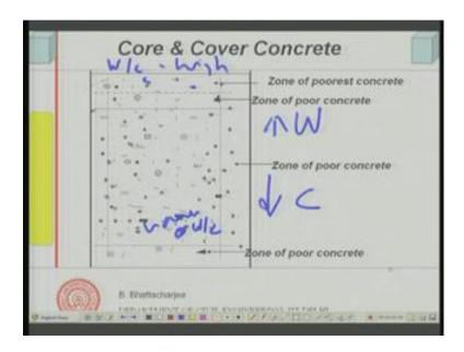
We can see if this is my concrete, this concretes these are the zone of poor concrete why, because this places the wall effect etcetera comes into picture. So, concrete is not compacted as well as this. Similarly, this zone again concrete will not be as good as well packed compact will let us say this point. But another issue is there; obviously, water cement ratio will be minimum here, because cement will have a tendency to come down and water tendency to come up.
