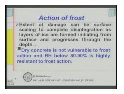
So, generally extent of damage starts from surface scaling, as we said from surface scaling right to complete disintegration as layers of ice are formed, initiating from surface and progresses through the depth. So, it starts from the surface and goes through the depth. Most important again, dry concrete is not vulnerable to frost action and R H below 80 to 90 percent. 80 to 90 percent is highly resistant to frost action.
