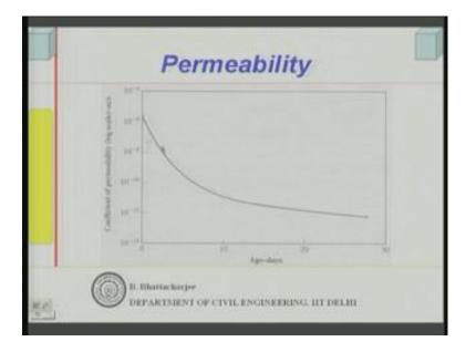
It has been observed that, with age the permeability would decrease. You know permeability coefficient of permeability in concrete decreases with age. This with concrete, that was with the you know this, I mean this cement paste. And similar all cement paste materials that behave in the similar manner. So, this is in log scale. It is actually it as the age increases. (Refer Slide Time: 28:25)
