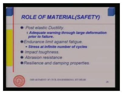
This is an important issue, post elastic ductility, post elastic ductility is an important issue. What is ductility? It is the capability of deformation. Prior to failure a formal definition would be given a little bit later on, but why do we need this? Adequate warning through large deformation prior to failure is required. I must know, that failure is, you know, I must get a warning for impending failure, so that I can do evacuation or whatever it is.
