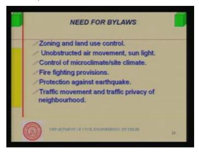
Well, one point I missed, that is, need for bylaws. Now, when we are doing functional design of building, certain restrictions are required to be put by controlling agencies because as I mentioned, the microclimatic modification is done by, by your construction, new carbon constructions, which we have provided that would change microclimatic conditions.
