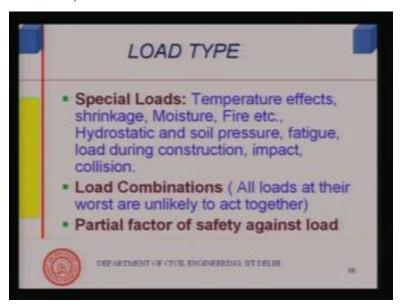
So first we did was, this is what we did. Load type, we looked into special loads. I mentioned, that temperature effects, shrinkage, moisture, hydrostatic and soil pressure, fatigue and fatigue load and also, load during construction, impact and collision, these are special loads. Then, load combinations is one thing, which one has to decide.
