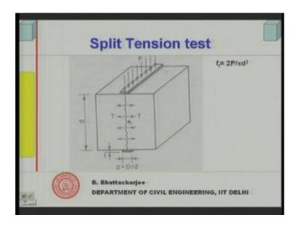
It can be done on cubes also it can be done on cubes also IS 500 and IS 500 and 16 allows it to do it on cubes or any other code allows you to do it on cubes. And this is how it is applied on a cube as well and the formula here is of course, slightly different it is twice P by pi d square, because we are calling this as d this dimension as d.
