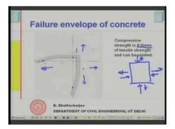
So, that can be understood from the failure envelope of concrete, you know if you remember we talked about bi axial testing of concrete. So, when we look into the bi axial. For example: if this axis shows the tension in a given x direction and this is tension in the y direction, in other direction bi axial situation we are looking at. This is the compression and this is also compression right.
