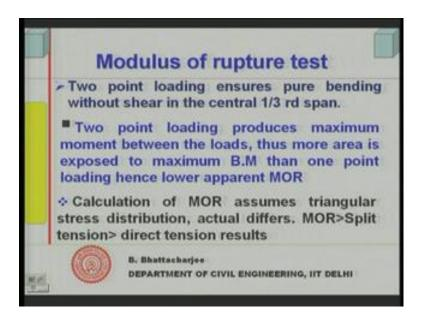
So, 2 point loading therefore, summarizing this discussion just now, I have talked about 2 point loading ensures pure bending without shear in the central 1 third span 2 point loading produces maximum moment, between the loads, thus more area is exposed to maximum bending moment than 1 point loading hence lower apparent modulus of rupture. So, when we compare between 2 point loading and 1 point loading we find 2 point loading gives us lower apparent modulus of rupture.
