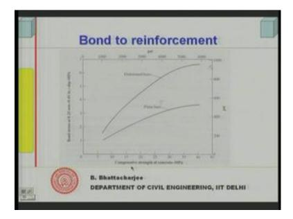
Last is the bond strength and bond strength of concrete again, can be related to compressive strength like this, bond strength of concrete can be related to compressive strength like this. You know, in this manner you can relate it to the compressive strength like higher the compressive strength, bond strength increases.
