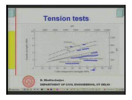
But this influence is not seen in case of other 2 that is direct tensile test and test for you know another is the split cylinder test. In split test we do not see this and this diagram shows us this behavior as we can see you see in case of splitting test splitting test both direct wet and dry is shown by this line. And which is showing least which is showing actually, least compared to all 3 splitting well wet and dry both are same.
