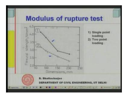
And you can see that in fact, people have tried to do the test with 2 point loading and 1 point loading and 1 point loading tends to give you always higher load 1 point loading always tends to give you higher load right.
