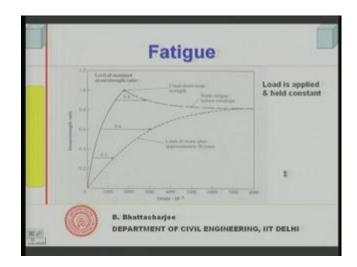
This is static fatigue this diagram shows you static fatigue. For example normal rate of loading as we have we know that 100 and 40 kg per centimeter square per minute that is what about 3 minutes, we go to failure and this is about ultimate short term strength, but if I go at a faster rate very faster rate I will get still higher strength, but if I slow down this rate, I have reached the ultimate short term strength you know in 2 minutes then my strength reduces.
