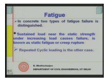
I said that there can be 2 types of fatigue behavior you know 1 is sustained load, it is not need be repetitive loading, but you have sustained load near the static strength under increasing load and this causes failure you know very slow rate of loading you have just load applied load near the near the static strength and its failure.
