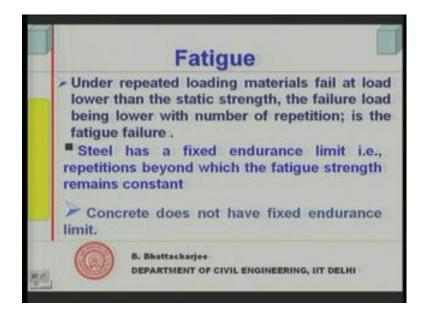
Let us look into now what is called fatigue what is fatigue well, in case of concrete we will define it in 2 different ways later on, but in general first define when you have repeated loading material fails at load lower than the static strength. The failure load being lower with number of reputations you know for example, supposing, I have a load I repeat go you know I start from a load and increase the load and bring it down.
