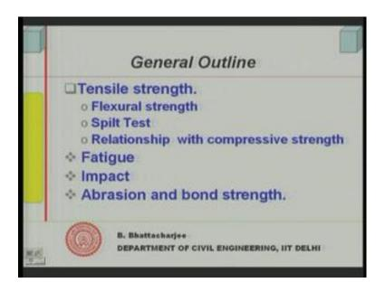
So, tensile strength we will look into first tensile strength of concrete and the general outline of our discussion today would be tensile strength. Now, we look to tensile strength in 2 different ways; one is called flexural strength other is split test. We will describe this and this relationship, with compressive strength that is what we look into. Then individually, we will look into fatigue strength, impact resistance of concrete and abrasion and bond strength.
