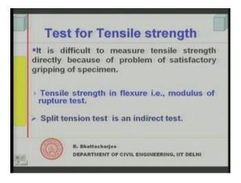
Now, how do we test for tensile strength how do we test for tensile strength? It is difficult to measure tensile strength directly, because the specimens you know initially
