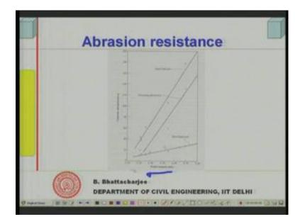
You see as the water cement ratio decreases as the water cement ratio decreases, as the water cement ratio decreases as the water cement ratio decreases the powder that is formed under grinding that is a measure of abrasion.
