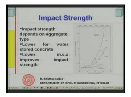
Next one is impact strength well. This is another issue important 1 impact strength of concrete, it has been observed that lower the water cement ratio you know impact strength depends upon aggregate type a strong aggregate would; obviously, show higher impact. For example some sort of you know angular aggregate this is granite this is gravel.
