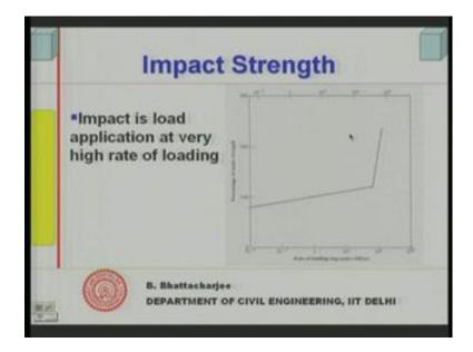
But actually means of very fast rate of loading. So, when you have very fast rate of loading the impact strength is generally higher than, the compressive strength that 1 can understand. So, rate of loading when it is very high that corresponds to impact strength and actually strength can be 200 percent higher right; last is the abrasion resistance and this also can be related to the compressive strength of concrete.
