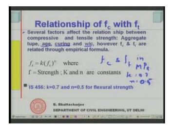
So, in case of in case of design we use specific value which has given in code. There are several sort of relationships are available. In fact, several factors affect this relationship these factors are something like aggregate type age curing condition water cement ratio.
