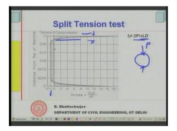
Now, let us look into the split test. This is the typical stress distribution across the across the across the diameter you know this axis shows 0 to D. So, this is the diameter of the specimen, this is the diameter of the specimen 0 to D and if you look at it this side beyond this point this point beyond this point compression we are calling it positive and tension is negative.
