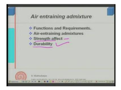
Now, the other kinds of admixtures which are also affect some amount of workability are the air entraining admixtures well. If you look at air entraining admixtures their main function is against freezing and thawing they show good durability performance against freezing and thawing. Air entraining agent essentially, improves the surface changes of surface tension of the water and thereby creates air bubbles.
