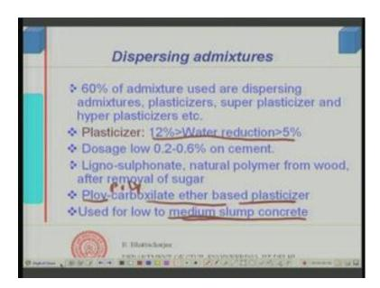
So, we are focusing our discussion on dispersing admixtures as you can see 60 percent of the consumption of admixtures, in the world actually 60 percent is the dispersing admixtures. That is majority of the admixtures are used for plasticizing or improving the workability of concrete or improving the workability of concrete just to little bit
