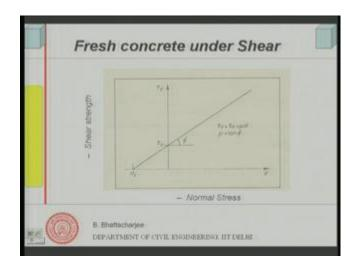
Now, follows from that is this relationship if I plot the normal stress versus the shear stress I get tau 0 here; that is at 0 normal stress this is the value of tau 0 and beyond that at higher normal stresses tau y and you know at any point yield stress is a function of tau 0 plus mu sigma. So, what do we see is yield shear stress depends upon the normal force as well.
