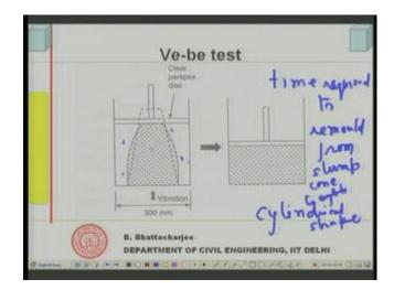
The third popular test is called Ve be test and this is as I told you, it is a original it is a modification of the original remolding test you know what you do is you have the same slump cone again. And on top of that you fix a perfect disk on top of that, so this is your original slump cone filled in with concrete in the same manner and put the slump cone here; remove the cone.
