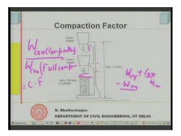
The next test which is quite useful in the laboratory and also used sometime in the site also, but then it must have site laboratory. Now, this is called compaction factor test so what, you do in this case? You actually have a hopper you know it is a truncated cone again, but it is a hopper right its bottom is closed.
