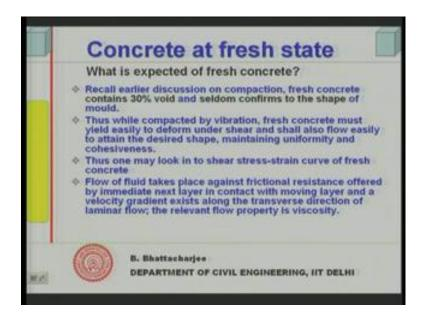
So, you can start with first what is expected of fresh concrete, if you recall our earlier lectures in 1 of the earlier discussion related to compaction we said that, fresh concrete contains about 30 percent pores voids and its seldom confirms to the shape of the mould. So, what 1 has to do 1 has to compact it to remove this voids and also; ensure a little bit of mobility, so that it moves it flows and then attains the shape of the mould itself.
