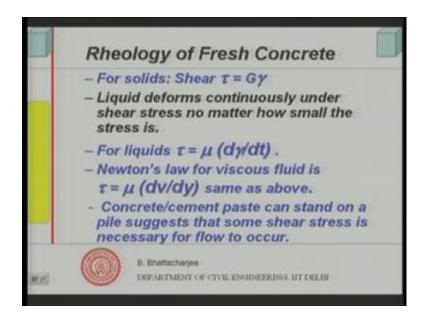
We will see that how 1 can model concrete with respect to these properties a little bit. You know for solids: shear stress is proportional to shear strain and if you look at fluid it deforms continuously under stress well no matter how small the stress is... So, solid does
