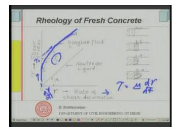
Now, let us see what happens in case of plastic concrete how does it behave. The plastic concrete is considered to be what is called a Bingham body. Now, if you see if you plot rate of shear deformation in fact, this should be d gamma dt rate of shear deformation
