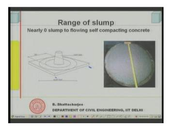
Now, what could be range of slump? Slump can very nearly zero to completely flowing self compacting concrete. Now, what is 0 slump concrete? Well, 0 slump concrete it is essentially meant for what I said roller compacted concrete. Now, roller compacted concrete may be discussed in some time.
