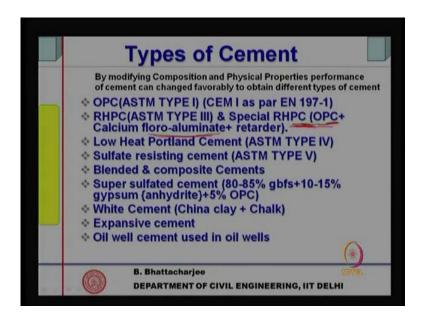
Now some special cement of this kind was is can be developed using composition of flora aluminates, you see special rapid hardening Portland cement can be generated with calcium flora aluminates and some sort of retarder. So, this is this reacts extremely fast and sets also very quickly and it is grinded to a very fine level.
