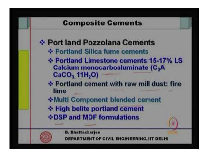
So, blended cements are blended cements are produced from this, one important issue is that such cements when, you produced by inter grinding gypsum clinker and the pozzolona, their strength initial strength is lower, but long term strength is better particularly with fly ash on. So, is the case with slag, but silica fume can show, you high early strength as well.
