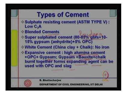
Now, this blended cements uses pozzolana a material, I might have mentioned earlier in the history when, I was talking in the introduction right. So, that is what so before that just expansive cement lets cover it up fully, high alumina cement with O P C and gypsum, because you see ettringite formation would occur with this one. High alumina cement and gypsum and this ettringite occupies more volume then the original reactant, therefore, it causes expansion.
