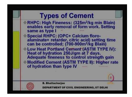
So, this cements we have looked into right, now we will go back to the first slide again. So, physically rapid hardening portable cement high fineness 325 meter per square k g minimum lengths enables early removal of form work setting same as type 1 as I mentioned. Special rapid hardening Portland cement O P C plus plus calcium flora aluminates retarder sometime, this retarder is the citric acid setting time can be controlled, it has got a very high specific surface.
