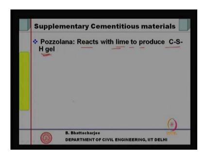
Now, this is what has been used for many many years. So, what we know is that some material some silica can react with lime to produce C S H gel like structure, you know lime with clay, that is what you say lime with contains active clay and reaction of clay and lime leads to cementing property. Now, this was actually discovered pretty early like
