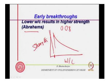
Then, I said that... What cement ratio used was 0.08 by D. A. Abraham. And, we also found that, strength is a function of water-cement ratio; in this manner, it reduces. Therefore, if I have high low water-cement ratio, strength will increase. And if you can pack it so well, you can get very high strength. Therefore, this was the understanding from D. A. Abraham's work.
