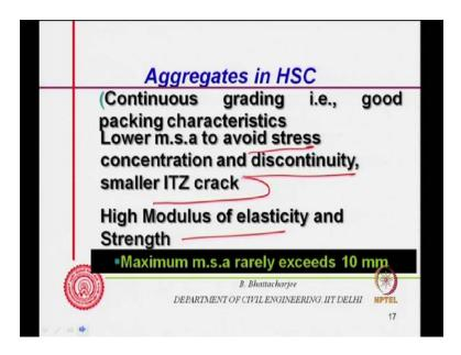
Now, what about the aggregates? I should have a continuous grading and good packing characteristics. Continuous grading means right from cement or silica fume size to the m.s.a, there should be a continuous grading. Now, this situation can well be understood; I will come back to this; I will come back to this.
