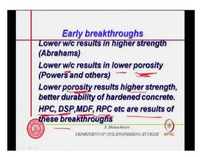
Therefore, the whole idea to get higher strength, I must reduce porosity. But, then, I also talked about – if you recall pore size, for the same porosity, smaller pore size will give you higher strength. So, reduction of the porosity and refinement of the pore sizes are important for high strength system. So, if you want to get a high strength system, then you must reduce down the porosity and you must also refine the pore sizes.
