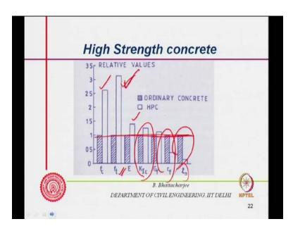
Then, this is modulus of elasticity – definitely higher. These are the fracture properties – the various kind of fracture properties; I will just define them. Some of the fracture properties, for example, energy absorbed will be lower; the length of the fracture, length around the tip would be lower. Some of those things are lower, which is actually sign of brittleness and so on and so forth.
