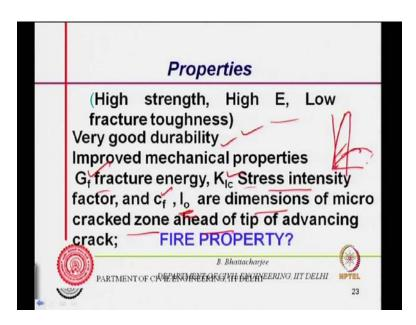
Some properties – strength obviously improves, tensile strength also improves; modulus of elasticity also improves not to the proportion of the compressive strength; but, it
