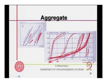
This we have already discussed – the particle packing. Therefore, quartzite concrete is somewhere here, stress-strain curve; standstone concrete is somewhere here; limestone concrete – stress-strain curve is somewhere there.
