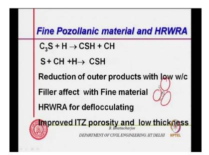
This is what the reactions we have looked into; typical C 3 S reaction would produce CH; and, this CH together with the silica fume will produce CSH gel. So, this is the secondary pozollanic reaction. This will be the case in high strength concrete too. And, this is essential. Of course, in normal concrete, you will have also if you add pozollanic material there. So, reduction in outer products with low water-cement ratio.
