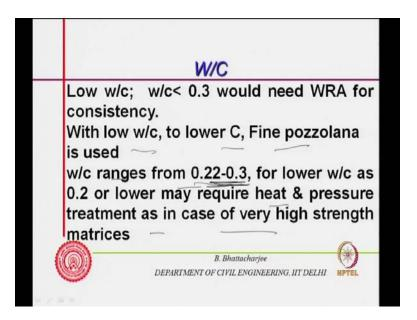
Low water-cement ratio – water-cement ratio will be less than 0.3. And, therefore would need water reducing agent for consistency. That we have seen. We have already said that, this is what we need for high strength concrete. So, what we are seeing – good quality cement preferably with low (( )) Then, water-cement ratio should be lower; and,
