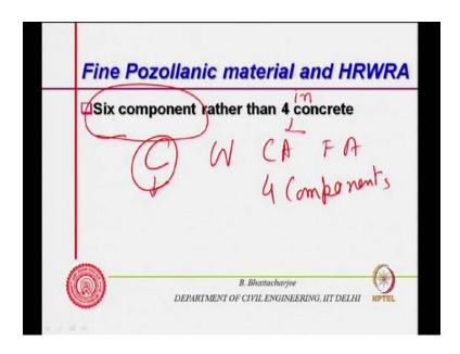
Now, that brings us to the situation that, actually, six component rather than four component concrete; six components rather than four in concrete; six component concrete rather than four; six component rather than four in concrete. So, basically, earlier, we are using cement, water, coarse aggregate, fine aggregate – four components. That is very conventional, very very old. Even modern engineered concrete of any
