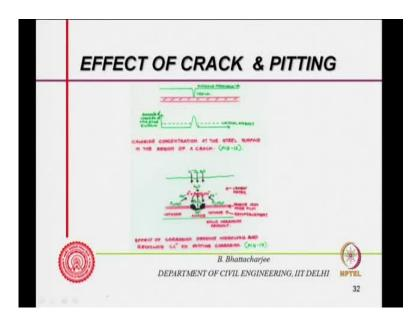
So, if you have a crack than chloride can penetrate and it can cause what is called heating corrosion that is what is shown here. So, with this we can actually summarize our discussion we have looked into carbonation and chloride together and as far as chloride is concerned we said that the c 3 a it gives better binding carbonation impervious concrete and low water cement ratio is better, and you know de-passivation time we have looked into some of the models and with this.
