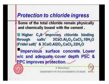
While slag cement is better both sulfide as well as chloride, so, higher c 3 implies chloride right and impervious surface concrete lower water cement ratio adequate cover depth t p c etcetera improves chloride. Threshold chloride depends on steel blended cement performs better and initiation period depends on steel type ratio as soluble chloride to water soluble chloride is this that is gamma values is something like this.
