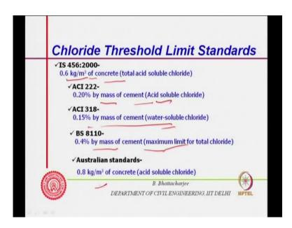
And therefore, you find that a various codes of different values you know for example, i s 456 you said this for r c c only 0.6 k g per meter cube a c i 220 0.2 0 by mass of cement acid soluble chloride 318 0.1 5 by mass of cement water soluble chloride, so, this is acid soluble this is water soluble b s 8 1 1 0 0.4 percent by mass of chloride and this is for total chloride, and Australia standard 0.8 k g per meter cube of concrete acid soluble chloride.
