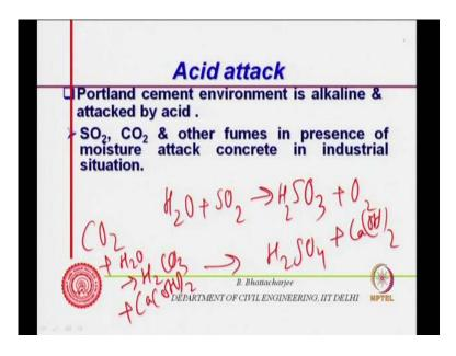
So, next we can look into acid attack, concrete is alkaline, port land cement environment is alkaline therefore, it will be attacked by acid. So, acid comes from where, sulfide dioxide, carbon dioxide in such other fumes if presence of in presence of moisture for example, you have H 2 O plus S O 2 will form actually h 2 S O 3 sulfuric acid which might get oxidized to you know which might form actually H 2 S O 4 you know H 2 S O 4 in presence of water etcetera, etcetera.
