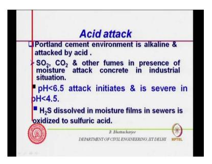
So, this is in in you know this is in in H 2 O dissolved in moisture films in sewer is oxidized to sulfuric acid. So, H 2 S, H 2 O plus oxygen in the atmosphere it is dissolved film it can actually results in formation of sulfuric acid. So, sulfuric acid you know this can result in again, reaction with the similar kind as we have discussed.
