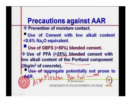
Use of ground granulated blast furnace slag or blended cement or fly ash, they actually reduce the alkali aggregate reactivity, the alkali use are alkali aggregate reactivity you know. So, blended cement because 50 percent the alkali content will get reduced by 50 percent, alkalis in the blast furnace slag or fly ash they do not contribute to alkali aggregate reaction.
