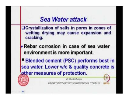
So, crystallization of the salt in the pores can occur and this can cause expansion and cracking. So, some slat pores will, it will become more, it will become porous, it will become porous this skeleton will become porous and therefore, more material can be go in solidified there and has the crystallization of you know solid occurs within this can cause expansion and cracking.
