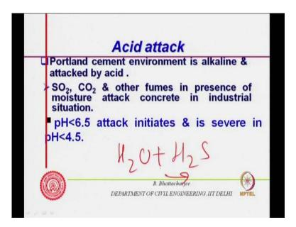
So, acid can attack concrete acid can attack concrete acid can attack concrete acid can attack concrete right. Now, p H below 6.5 attack initiates and a severe if p H is 4.5. So, concentration of the acid matters, sulfuric acid I mean the formation of sulfurous acid or similar one or C O 2 carbonic acid if it if it concrete come soon in contact with p H less than 6.5 attacks initiate and it is very sever in 4.5. So, it is actually cause lot of loss of the material from the concrete itself.
