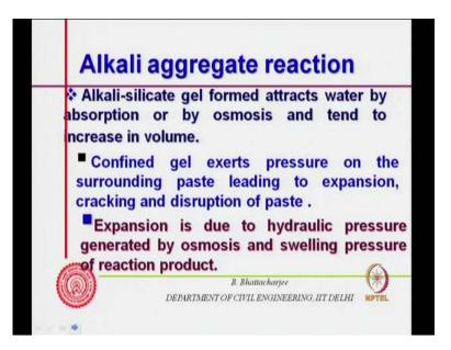
And once they attract the water, they tend to increase in volume and volume expansion you know, this volume expansion of this confine gel tends to exact pressure on to the surrounding paste leading to expansion, on cracking and disruption of paste, leading to expansion and cracking and disruption of the paste, right doing to expansion and disruption of the paste.
