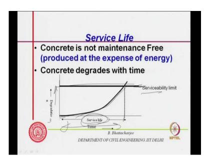
So, it will have a tendency to react, concrete will some component of concrete particularly cement systems, cement hydrates system that was not dissipated it is energy fully and therefore, it will have a tendency to react. Aggregates actually if it is fine powder, then you know like after a brush on natural process fine sand, very fine sand, large sizes also has got to reduced.
