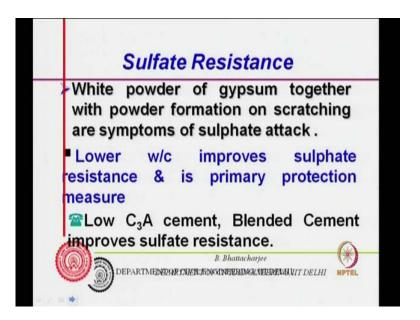
Now, how do you reduce it down if you are, you know if you forcey the sulfate attack, then lower water cement ratio is a good solution, it improves a sulfate resistance and it is primary protection measures. So, basically you have to reduce on the water cement ratio what it what it is sulfate will not be able to penetrate into to the concrete, sulfate will not be able to penetrate into the concrete, you know as we said moisture has to come in the other material has to come in to the concrete.
