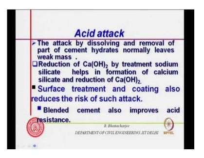
So, surface treatment and coating also reduces the risk of such attack, even even you know even even water pure water 7 p H water, you know distilled water they have a tendency to actually leach out because leaching from the concrete. So, concrete close to neutral or less than neutral that is acidic water, as a tendency to actually become more porous and in the process they can be, they can form weak mass.
