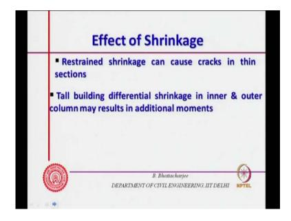
Cracking can be measured by ring test that is what I just mentioned you can go on recording this. So, this is what is the, you know ring test from which you can measure. Now, what is the effect of shrinkage? Effect of shrinkage is restrained shrinkage causes can cause cracks in thin section.
