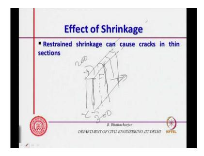
For example, if you have a wall if you have a wall you know a wall like this thin wall thin wall and is restrained construction joints are not given have not been given let us say. You might find cracks like this, you might find cracks like this at regular spacing
