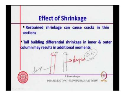
High strength concrete are susceptible to autogenous shrinkage high strength concretes are susceptible to autogenous shrinkage, because you have lot of cement past in the system. And therefore, there may be you know susceptible to shrinkage. So, one has to see that one has to you k therefore, this is studied for low water cement ratio system
