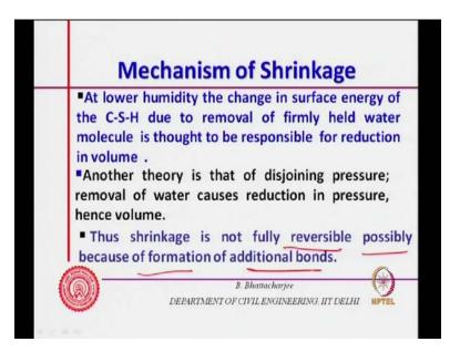
So, this is another reason there is collapse mechanism sort of. So, this results in adsorbed water removal can cause actually change in the volume or shrinkage. So, this is another theory.
