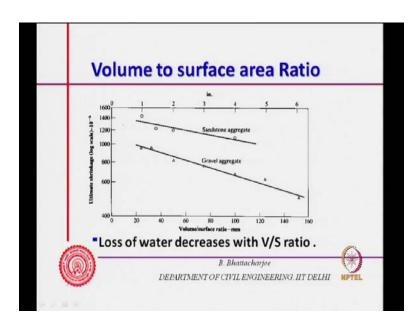
So, loss of water decreases with volume to surface area ratio with increase in volume to surface area ratio; that is the idea.
