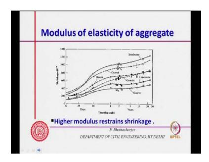
So, higher modulus restrains shrinkage; that is what we are saying, higher modulus restrains shrinkage.
