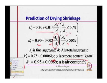
We can look into k 5. k 5 is related to fines to coarse aggregate ratio. So, equations are given again. If the fine to coarse total aggregate content is less than 50 percent; in other words if my fine content in the concrete is less than 50 percent, alright. So, equation is here. If this is more if more fines are there more shrinkage; if lesser fines are there less shrinkage, because coarse aggregate is the one which will actually restrict the shrinkage.
