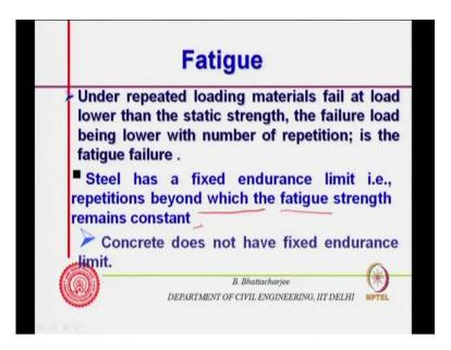
But, beyond 10 to the power 7 cycle or some cycles slightly above 10 to the power 6 cycles and 7 cycles you know. The endurance the fatigue the load at which reversal this is occurring at 0.4 or so close to 0.4. So, around you know like 250 mp is the yield strength of mild steel if endurance limit is around 100 close to 100 mpa. So, that means if you apply less then you know 100 mpa and do stress reversal actually it is not going to fail.
