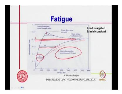
And this is again strain versus stress graph. So, limit of strain after approximately 30 years. So if I look at it static rupture curve is here maximum strain after 30 years this
