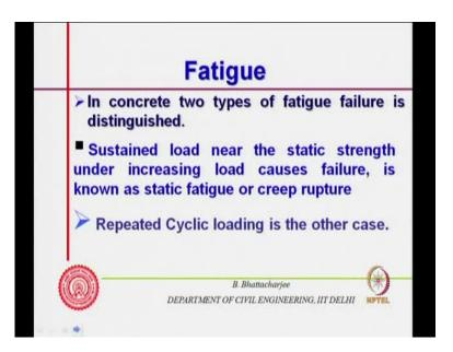
So, this is how we define. Now in concrete 2 types of fatigue failure is distinguished the one if a Sustained load near the static strength, under increasing load causes failure. So, its static fatigue or creep ruptures.
