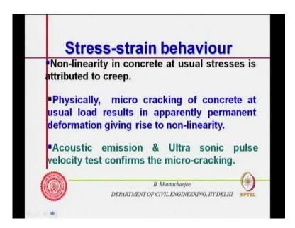
Now, this has been confirmed by test such as acoustic emission and ultrasonic pulse velocity test. So micro cracking is generally confirmed by this. Now, let us see let us look at this, so you see if I look at if I applied load like this. You know if I apply load like this whenever the specimen is here, if I apply load like this specimen is here if I apply load like this. Now, this is longitudinal strain that means strain along this direction, the strain along this direction dimension change.
