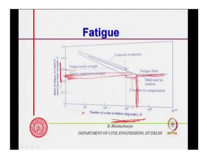
If you look at this diagram on this axis number of cycles drawn in log scale. Because, 10 to the power 2 etcetera this is log scale and ratio of the fatigue strength to short term static strength. So, actually if you are operating at you know fatigue strength you will find that in case of steel, this is mild steel in tension you do reversal of stresses.
