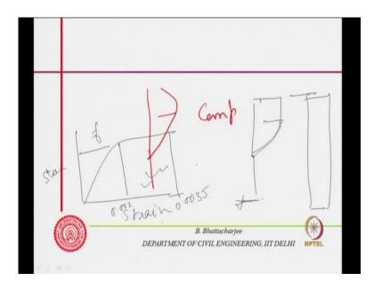
Therefore, one should be using this sort of curve and compression you know. So, this is if you remember flexural design flexural stress strain curve given in the code would be something like this. You know stress concrete stress strain curve of concrete if you recollect this is strain inflection, you know if, it is a beam section of a beam if I am looking at a section of a beam this is a reinforcement this is the concrete, anyway.
