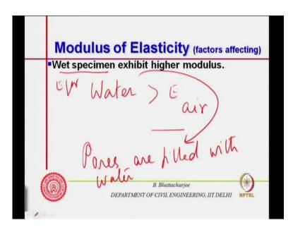
So, first thing is this other factors which specimen exhibit higher modulus why because water has got E for E for water for water is more than E for here both are fluid by the way. So, wet specimen the pores are saturated with water. For wet specimen pores are saturated with water pores are filled with water they replace the air. So therefore, modulus of elasticity it is likely to be higher.
