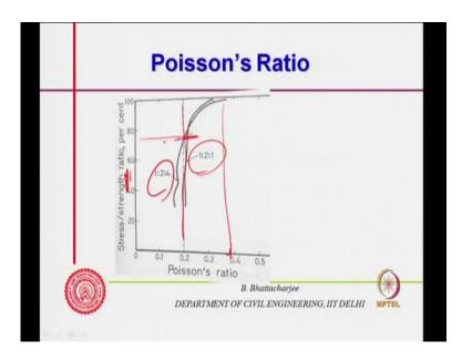
Now, mu values if we calculate out in this manner and then plot, we will see that which is roughly around point 0.2 it is roughly around point 0.2 up to about 70 percent of the load for 2 different concrete good old days people conducted experiments and found out. But, beyond that point actually it starts increasing it starts increasing can go close to about point 0.3 or so on so forth.
