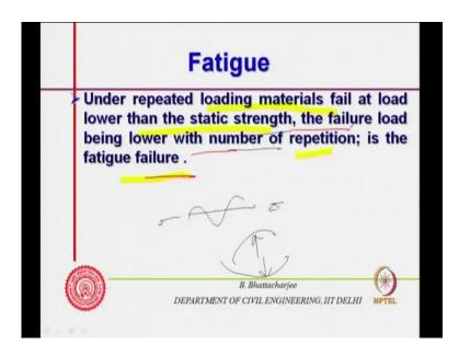
But, if I try to bent it in this manner that means bent it in this manner you know reverse is the stress. There is a reversal of stresses so you bent first you bent it in this manner then bent in the reverse direction. So, first you bent it in this manner then reverse direction you go on doing this after sometime it will break. So repeated loading you can you know it fails at much lower load and that is basically much lower load and that is basically a fatigue failure therefore.
