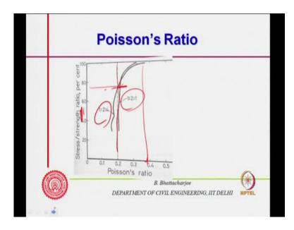
With the you know like if your stress to strength ratios, so when before failure, so before failure Poisson's ratio increases and we understand this. Because, lot of micro cracking would have occurred and that would have caused lateral strain to expand you know increase it at a faster rate than the longitudinal strain.
