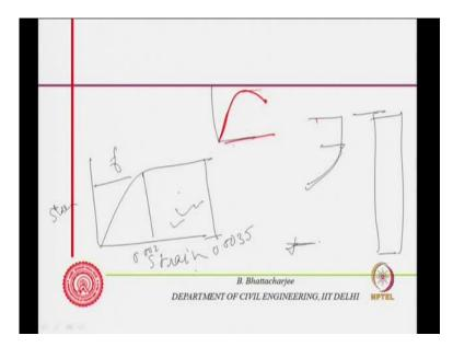
Stress strain of concrete will look like this maximum stress and here. Now, this is idealized stress strain curve beyond that you assume is as if it is straight line. So, actual stress strain curve of concrete will like this and this is important in flexural design. So, this measured stress strain curve that we have seen.
