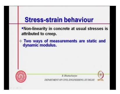
Now, that is called dynamic modulus so dynamic modulus is related to dynamic modulus is related to wave propagation within the material itself. Because velocity of wave propagation or characteristics you know wave propagation is related to elastic modulus and one can determine that wave.
