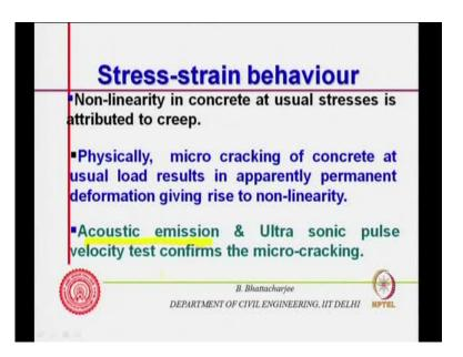
So, this is Acoustic emission we just mentioned about acoustic emission emanate. Before we mentioned that you know you can we, you do acoustic emission acoustic emission and ultrasonic pulse velocity confirms micro cracking.
