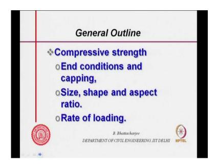
You know such a factor those will be affecting the strength. So, general outline compressive strength. The factors which affect the compressive strengths are end condition and capping of the sample or the specific, you know sample of the specimen that I take, size and shape and aspect ratio of the specimen rate of loading, and then will look into some of the aspect related to tensile testing some of the aspect related to tensile testing.
