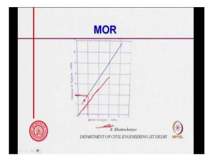
So, what is split tension test? Split tension test this is what it is tensile strength modulus of rupture you know this is of course, direct. So, this in linear of course, they are linear, but this is always lower you know this is not line here not this is somewhere here. So, when this is one this gives you somewhat higher value. So, this direct tensile strength or tensile strength is pretty lower.
