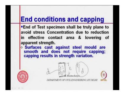
Now, end condition and capping, end of test specimen shall be truly first of all you know it should be truly plane, this is what we talked of now this should be truly actually, this should be truly plane, this portion should be truly plane, this should be truly plane. Otherwise, the undulation the contact area would reduce, and there will be stress concentration, you know effective contact area will reduce, and apparent strength will reduce.
