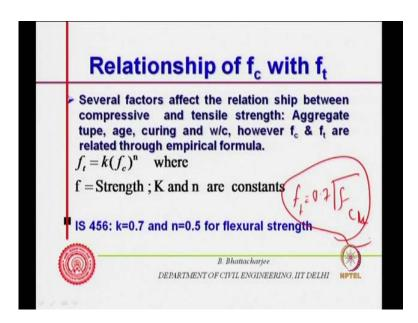
So, several factors affect the relationship between compressive and tensile strength of aggregate, you know it is aggregate type, age, curing, water cement ratio. But, through
