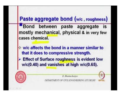
So, it is mechanical bond you know mechanically you want to pull out, this is the paste so it is it could be mechanical bond sitting on the roughness of the aggregate. Physical between the paste to paste is physical, paste to aggregate is you know not necessarily not not not many times physical bond. But, adhesive forces can exist because you know one was in plastic state, other is solid, the aggregates are generally solid, paste was in plastic state.
