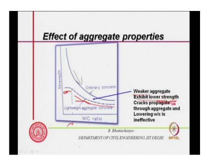
So, strength is usually governed by the weakest link, if the paste is weak and paste ITZ is weak, it will pass through ITZ, it will not cause cracking of the aggregate but it may start from ITZ in any case, if it is a largest void. But, as it initiates, it might pass through the aggregate straight way if the aggregate are weak. For example, if you just bricks low strength bricks something like 7.5 mpa or bricks or 10 mpa bricks and crush them and make aggregate out of them.
