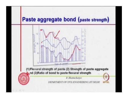
And to do that, one can look into this kind of a diagram, which shows said that figure this one this one you know this one shows diagram 1 shows, if we have different cement, the flexural strength of paste would be something like this flexural paste strength of paste would be something like this flexural strength of paste. Two shows, strength of paste aggregate bond two shows strength of paste aggregate bond so this is the paste aggregate bond you know.
