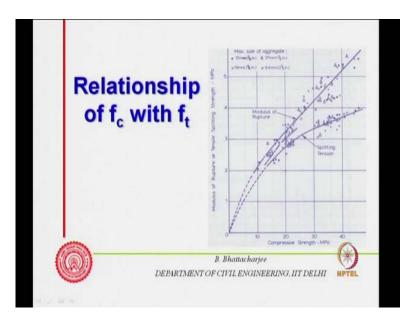
Some equations have been developed and several factors of course, will effect this relationship, as we have seen in the previous curve as we see in the previous curveyou know. The type of aggregate the scatters is because of the type of aggregate, m s a values and maximum you know m s a values and there could be other cases such as moisture condition, etcetera, etcetera many factors would affect this.
