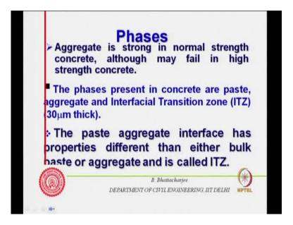
You have got ITZ the paste aggregate interface has properties differ then either bulk paste or aggregate and this called ITZ. So it is different when the bulk paste itself it is different when bulk paste itself or you know aggregate itself. So, it is different in paste and aggregate and it is, that is why we call it defines it almost as a separate paste. Now, why it is we can be able to actually understand gradually will be able to understand it gradually.
