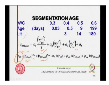
So, just let me put it in words now, let me put it in now words, you see what we have seen the r point 5 r point 5 is a function of r point 5 gel to the some gel porosity. And it is a function of water to cement ratio and age. Similarly, r point 5 capillary is also a function of water cement ratio and age. And we know the porosity itself is function of water cement ratio. So in other words what we are trying to say qualitatively quantitative we leave out.
