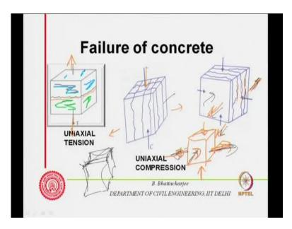
So thus have the mechanism of failure concrete and this you can understand. Supposing, I applying tensile load to concrete it should ideally fail Uni-axial tensile strength ideally
