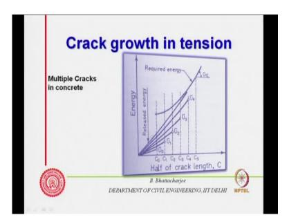
So, in other words this you can think of in terms of if there are you see this is the critical stress sigma T elastic modulus energy required to create a new surface. And this is crack length you can say this is a crack length of the elliptic crack. So, it is under tension this is under tensile force these all it will behave in other words this place a major role. So, if
