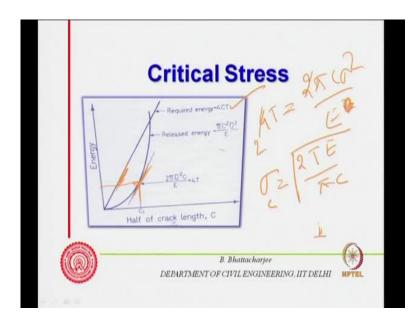
So, if I take this force if I take this rate of strain energy release this is the situation rate of strain energy. So at this stress at the stress corresponding to this point is a critical stress. So therefore, you can actually by E this is your this is by E square this is by E. And therefore, you can find out sigma is equals to this will be 2 so 2 TE divided by this is cancelled out pi.
