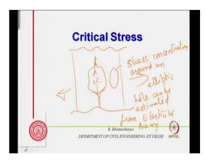
Supposing, I have got a surface something like this, there is hole and this is my material there is a hole. And I am pulling this material from this side, then what will happen, this crack will try to spin. Now if this crack tries to expand or, this hole expand the fracture propagates along this direction. So fracture propagates along this direction that means it creates new surface is here. Now this stress around a hole for an elliptic hole 1 can
