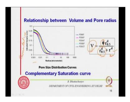
Let me say this is cumulative porosity can be related cumulative porosities from small pore size to other pores porosity. Can be related to porosity cumulative porosity, can be related to pore size and mean through in terms of mean distribution radius and over all porosity.
