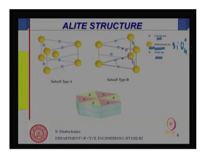
So, less look further into this cerotic calcium silicate hydrate or alite structures. This is got subsoil, if this is you know this one are the calcium irons, ortho silicate iron that is S i O 4, this is S i O 4, negative ortho silicate iron, oxide iron and calcium iron, they are arranged in subsoil's like this.
