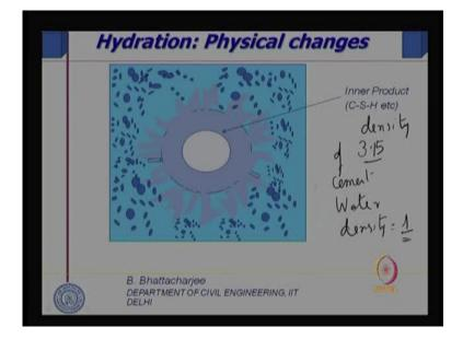
If you look at hydration process of you can consider small position of water like this, you know water like this an lets this is cement grain, cement grain as you know cross product is grinded. Therefore it will not have a rounded shape, it will have some sore irregular shape as we can see. So, it will have some sore irregular shape I can idealize this as a circle something like this right. So, cement shape was something like this idealize circle, now let say hydration proceeds.
