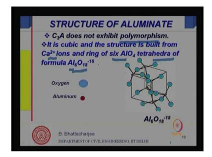
It has got one difference, it does not exhibit polymorphism it does not exhibit polymorphism. So, does not exhibit polymorphism, it has got a cubic structure of Al 6 O 18 with iron with 18 negative valiancy. So, cubic structure is built from calcium iron, it
