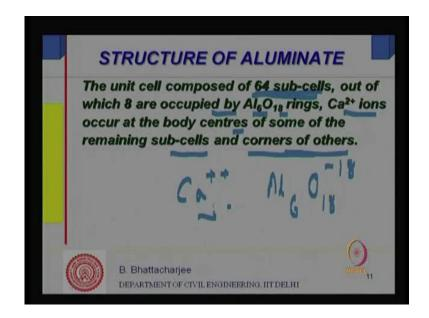
Now this is connected to calcium iron, this connected to calcium iron in case of Alluminate. So, you needs shell actually is compose of 64 subsoil's out of, which 8 are occupied by A 1 6 O 18 brings and calcium irons are you know, they occur at the body centre of some of the remaining subsoil's and corners of the other.
