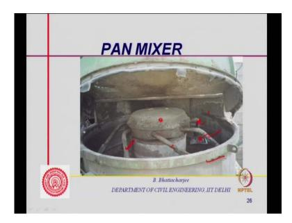
Scrappers this is the scrapper; there is an inner scrapper which you could have seen before, inner scrapper you know which will look like this; inside scrapper is the inner one, this is the inner one is the scrapper.
