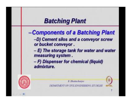
Then you have you know continuing the components, cement silos and conveyors screws or bucket conveyor for transporting the cement from the silos because you got to take it to the balance and then from balance to the mixing mission. Then storage tank for water and water measuring system; if you have admixtures chemical administer some kind of a dispenser for chemical admixtures which will actually add to the system before mixing, so this is the components.
