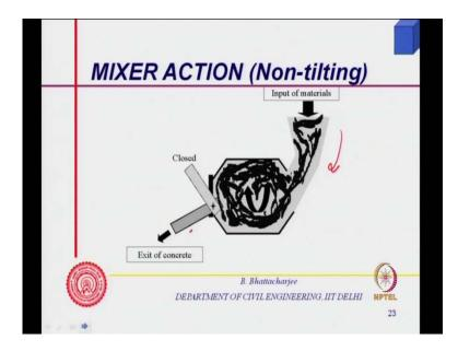
This is the non-tilting type; you feed it, this is closed, and when you want to discharge you can just open this, there is a shoot here. So, this is the feed of the material and that is how actually this is this is your non-tilting type you know mixture not very common.
