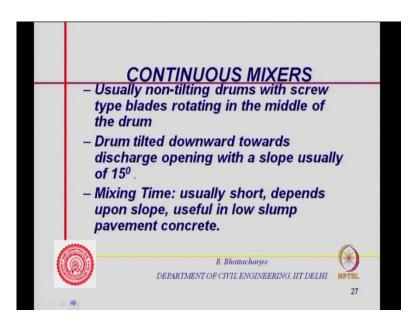
So, if you are producing large quantity of concrete this might be useful one. You feed from one side, and then it is a continuous batching also continues mixing also feed from one side and the screw type of blades that causes the mixing as it rotates the rotating drum rotates, and then it discharges at the end by the time actually the mixing has been finished.
