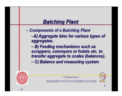
So, feeding mechanism is the next one. Then you have balance of measuring system for the aggregates particularly and also the cement.
