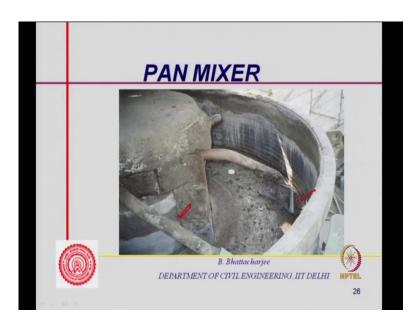
And then you have got the scrappers again outer one and then finally. So, you have inner scraper here and scrappers there. This is where the shaft, pan is fixed in this particular one pan is fixed. So, this is one type scraper, this is other scrapper; the smaller scraper you can see somewhere up there, you know this is other scrapper, this is the other scrapper, this particular one is other scrapper.
