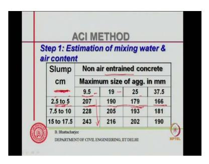
Having done that next is the step 1 part of it which will be you know actually step 3 in the ACI Method or else ACI report to 211, but here I am calling them as step 1. So, that it is actually estimation of mixing water estimation of mixing water. And, that we do from a table which is given below; that we do from a table which is given below.
