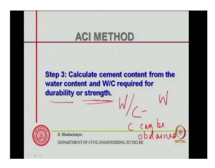
So, the next would be calculate cement content from the water content and water cement ratio required for durability or strength. Well, durability again controls water cement ratio is controlled you have a maximum limit of water cement ratio you have a maximum limit of water cement ratio. So, therefore durability is again controlled durability controls the water cement ratio. So, you have maximum water cement ratio and from the strength
