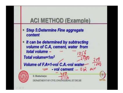
So, coarse aggregate content straight away you get it you get it. You know course aggregate content in 1 meter cube 66 percent of the material cube is actually occupied by course aggregate in bulk in bulk. And, therefore, I multiplied by bulk density; which means that there are force inside and rest of the material will be other material.
