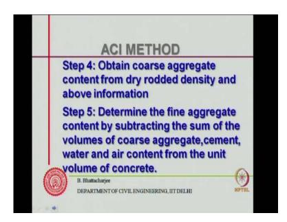
So, obtain course aggregate content dry rodded density and above information that percentage that you have got. And, then determine the fine aggregate content by subtracting the sum of the volume. So, course aggregate cement, water and air content from the unit volume concrete. So, than again it uses a conservation of volume concept. And, you can determine the total determine the fine aggregate content and thus how you got the proportion. So, you have got the proportion.
