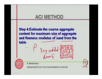
But here what is done is you find out the dry rodded density of the aggregate dry rodded density of the aggregate. That means, what you do? You have you pick the aggregates course aggregate in 3 layers aggregate in 3 layers. And, find out because volume of this is known, how much is the mass? This volume you can find out first by filling it water volume of the container. Then, put the aggregate then put the aggregate and find out how much is the mass of the aggregate?
