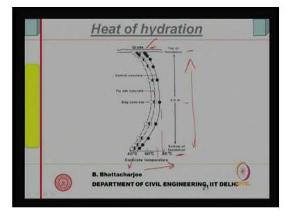
So this is 265 OPC this is OPC 265 plus 150 k g of you know this is flyash is 150 and ambient condition is here ambient profile the relevant ambient profile in two cases this is what is shown. So, actually temperature rise is much less when you use flyash and this diagram also shows the same thing for example, this is the top surface of a you know grade level top of a foundation.
