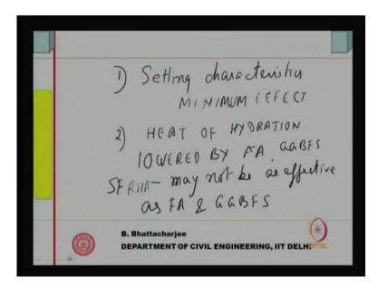
Using them right so this as far as their behavior in fresh concrete is concerned so what we have seen is number one we have seen that to start with they do not effect the setting characteristics setting characteristics minimum effect heat of hydration lowered by flyash and GGBFS but, may not be may not be.
