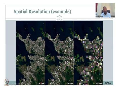
Some examples of spatial resolution, you could see it depends on the sensor it depends on the satellite payload. So, you have 300 size 130, So as the size goes smaller, the pixel size you could see more detail can be seen. So, 300 is too big, and within that just one colour is there, so you do not see much difference between houses and stuff. Then 100 meters per pixel. You can see some features coming up. But when you bring it down to 30 meters per pixel, you see a lot of more features.
