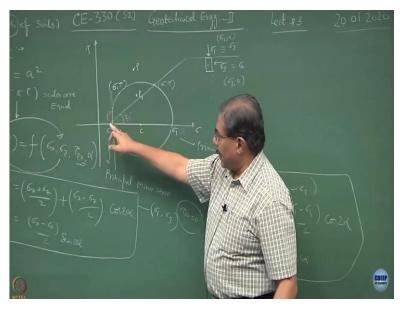
Where is your guess? Where the pole is, pole we have already identified.  $35^{\circ}$  line if I draw, this is the place where  $\sigma$  and  $\tau$  is acting. So, by definition, the state of stress has given me pole and pole is giving me a plane which is cutting the Mohr circle where the state of stress is to be identified. Is this part clear?
