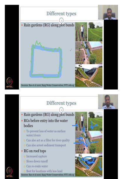
What are the different types? There are multiple multiple types of these, nature-based rainwater harvesting. Basically, it is a thick soil, on top of which there is a plant and the plant and the soil are acting together to slow down the water and infiltrate. So, first slowing down is done by the plants and then the root zone and the soil are in a particular fashion like mulch or treated soil which can actually increase the movement of water.
