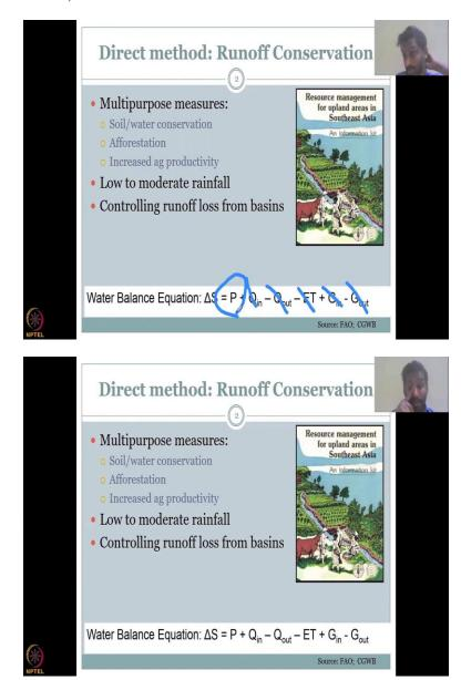
In the last lectures, we looked at how the methods are devised, it is direct methods, indirect methods, and a combination of both. In today's lecture, we will look at the direct method and most important methods for India. The first one is the runoff conservation. As the name suggests, runoff is from your water balance equation, we can get, which is the water which comes from rainfall, which is not going into the ground as groundwater recharge or storage, it just goes on the surface as runoff.
