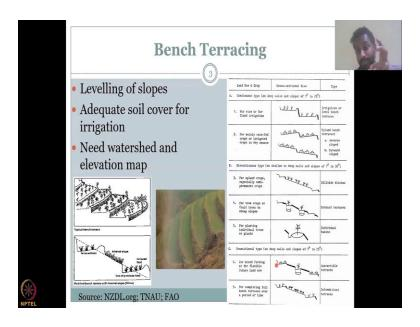
So let us look at some methods. The first method is the Bench Terracing. I am using the methods given in the CGWB manual, and I will be taking some references from TNAU, FAO et cetera. So what you, he here, have his bench terracing or, terracing is converting a slopy land into terraces. You cut through in between so that you slow down water.
