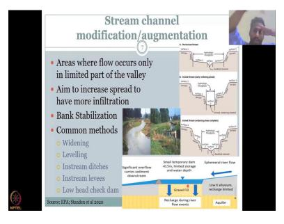
The next one I would like to touch upon is modification. So a modification of streams channel and augmentation is also very necessary for successfully reducing the runoff, and conserving the runoff for recharge. So what does it mean? So here what you see from the EPA book is that when a river is flowing, when a stream is flowing, when a water runoff is flowing, if it is made to flow in a very concentrated way, then fast, it will go and less recharge is happening.
