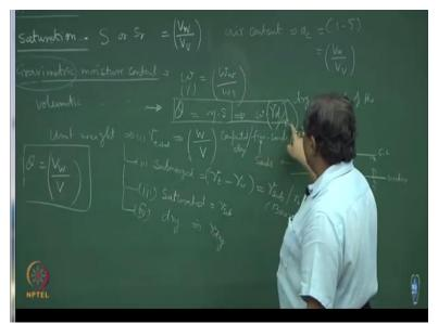
So please make 2 corrections gamma d upon gamma w into moisture content which is gravimetric and Vw upon V. Now let us go into the gammas, what is gamma total.
