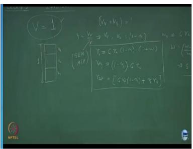
Here what has happened is, this 3 phase system if you remember with which we were working V air, V water, V solids this whole thing has been treated as unity. So I am doing now calculations which are volumetric, volume centric you may say try to prove that gamma = g into gamma w 1 - eta into 1 + w. So gamma dry = 1-eta into G into gamma w and what about the saturated thing G gamma w 1 - eta + eta into gamma w, first one is yeah this is gamma total.
