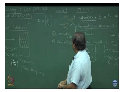
Suppose there is a soil mass like this, this is the ground level and I want to find out what is the total unit weight of the soil at point A there are several techniques. One of these techniques is you know we call it as a core cutter method. I am sure there is a laboratory experiment on this you must have done this, what normally we do is we make a small hole over here on the ground alright scrape out this soil, remove this soil put it in a polythene bag, so that the moisture does not get lost.
