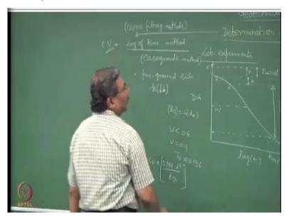
Please refer a book to understand the different aspects of the geometry which I have done over here, that would give you a better idea about how the construction is done. The second method is the known as the square root method, a square root of time method. So this is the first method of curve fitting to determine the C v value.
