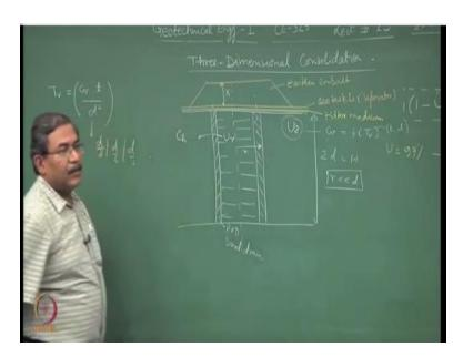
This is normally achieved by inserting the sand drains or sometime we call them as PVDs alright, pre fabricated vertical drains.
