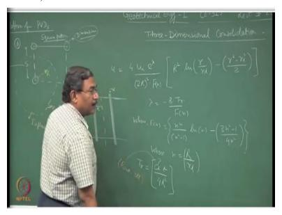
So the pore water pressure is defined as 4 u i e to the power lambda upon 2 R square into F n, F n is the function, R square into log of r by r d – r square – r d square upon 2. So this is the function which gives you the value of the pore water pressure where lambda is equal to -8 T r, T r is nothing but the coefficient of radial consolidation T v we have used for vertical consolidation upon F n.
