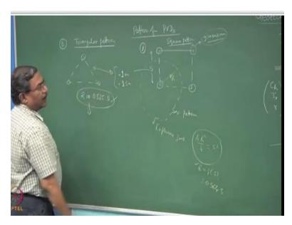
Normally what we do is we fix S center to center spacing is fixed as 1 meter, 1.5 meter, so S is known, R is known. Once R is known we will proceed further, the second pattern which is normally used to install the PVDs is triangular pattern. So this is a square pattern and this is the triangular pattern, again the spacing between the 2 PVD is less and get the value of R this turns out to be 0.525S, yes.
