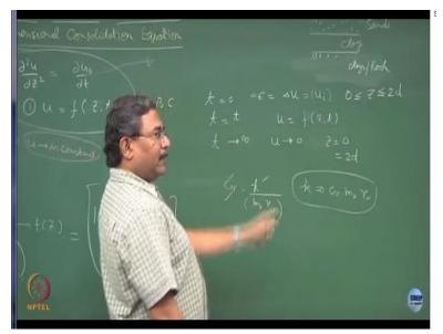
So C v = k over m v into gamma w alright, if I know the hydraulic conductivity of the soil, if I know it is m v value which I can obtain by conducting the one dimension consolidation test gamma w is known, C v can be obtained simple method. Normally this is not done we never obtain C v like this, what we do is, we obtain C v we knows m v, we know gamma w, we compute k. So k = C v into m v into gamma w hydraulic conductivity can be obtained by knowing m v value, C v value and gamma w.
