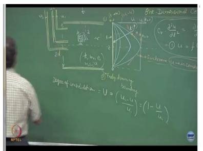
So that means if I want to plot let us say, this is z and suppose if I plot pore water pressures, so in the initial condition, what is going to happen is the value of pore water pressure which is developing air as well as air is going to be a constant, I hope you agree with this. So this is what is equal to u i, the moment you applied the pressure, the pore water pressure = u i at t = 0, now what is going to happen.
