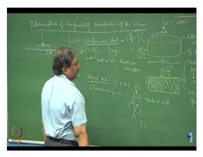
There are 2 ways. The first method is which is known as Oedometer test. We call it as Oedometer test, find out what is the meaning of the word Oedo. So, this is the hollow ring of stainless steel, normally 75 mm in diameter and 25 mm in height and made up of you know about 0.5 mm thick metal. Now, this is the odometer ring Oed is basically a sort of happiness. So, the name is a interesting name, this is what is known as a Oedometer ring alright.
