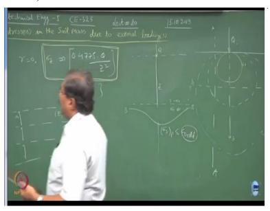
This is the ground surface at a depth of z, if I create a plane this is a plane at which I want to see the variation of sigma z as if you are cutting all these pressure bulbs along this axis. So if there is a plane which is passing through this, is the same plane as what I am showing over here. So the pressure distribution would be like, why the wetting takes place of the pavements, this is the answer.
