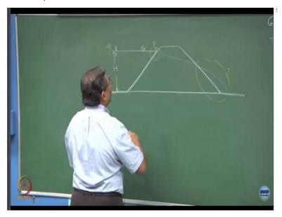
This is the upstream side of the water of height H ok. This is the equipotential line and this line is also an equipotential from the end point to the point where I have taken Y = H alright, that is how I think I created boundary conditions yeah. So from this point, this is a cos alpha and then I am substituting the value of a as this thing a sine alpha Y truly speaking, like this is an equipotential line the top phreatic line should have been perpendicular to this.
