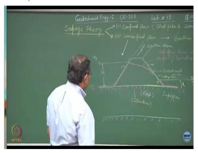
By definition, the unconfined flow is occurring in a situation like this, that if I consider an earthen dam. So this is an earthen dam it is a cross section in fact, is a embankment, we can call this as an embankment also. This is a third dimension which is going up to the infinity into the plane perpendicular to the blackboard. Normally we define the slopes as 1: m and 1: n, where 1 is vertical and n is horizontal.
