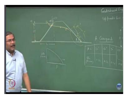
As you rightly said, the flow line is going to be perpendicular to the equipotential and not starting from this point, where the water is matching with the body of the dam it will be at a certain distance x. So the top phreatic line would start like this ok. Now this is near perpendicular then what will happen, this will go further down at this point where is the outcrop point now, outcrop point should have been somewhere here.
