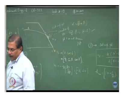
So if I substitute this over here I can show that sine alpha = sine beta cos delta. And if I substitute the terms I will be getting sine of alpha - delta = sine of alpha, what this indicates is that delta tends to 0, number 1. If delta tends to 0 that means, the discharge velocity at the free surface is going to be equal to whatever the V component is. So this always parallel to the downstream slope, this solution is valid when we say alpha is less than equal to 90 degree
