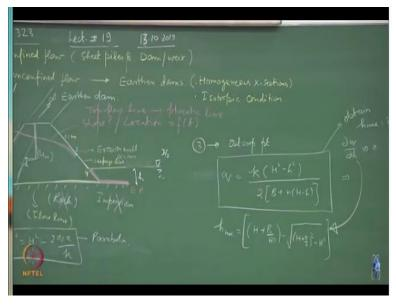
So what I can do is, I can write this expression as Q = k H square - h square over 2 times B + n H- h, this is a function which I get, is this part clear. So for a given H and a small h this is the flow regime which is getting developed. Now I want to optimize this function, so obtain h maximum. So if you differentiate this function and put it equals 0, what you will be obtaining is,
