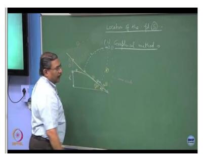
So this is the point s, one of the simplest method is you adopt the graphical method, please follow the steps which I am to going talk about. If this is a downstream side of the slope, I have taken this as alpha, what we are interested in finding out is the location of this point which is s and this is the height. This is the height of the water column let us say h or whatever the first step is extend this in the vertical direction and let it cut the downstream slope.
