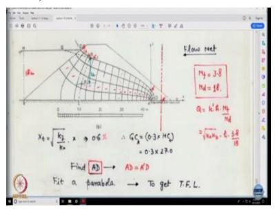
Because hydraulic conductivities are different in x and z direction, what we will have to do is we will have to go for equivalent hydraulic conductivity which is root of k x k z, what is causing flow h, h is known as 18 meters. So this 18 meter is going to cause the flow, after the flow net is constructed, I can count the NF and ND and this is 3.8 and 18. This function is transformation of x into x d direction, so root of k z by k x would be 0.6 times x.
