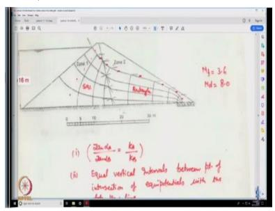
The last thing which I want to discuss regarding the unconfined flow is most of time we come across a situation where we have different zones in the embankments. So suppose I want to reduce the you know seepage which is taking place through the body of the dam. So there are 2 ways, one I did is by maximizing the h value and getting the value of Q, which is the inverse process.
