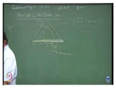
You will first lay in this portion, sudden layer of granular material you will start laying the soil on this side and compacting it. So this is the soil, second layer of soil, second layer of gravel or sands and then you can give it a shape of the final embankment like this. So this becomes my drainage layer and point A get shifted inside. Now the moment I have done this type of a manipulation the top floor lines will always come and cut at the vertex, so this is the vertex point E fine.
