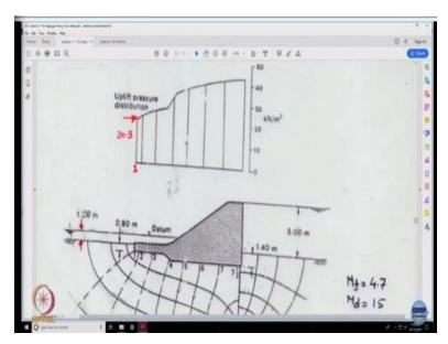
If you remember, when we were talking about the seepage force computation, I had drawn a figure where I had created a earthen dam. And then at the base of the earthen dam I had shown you that is a seepage pressure which is acting. Suppose you have to find out the pore water pressure at point 1, 2, 3 and so on. Now, this is a pore water pressure which is acting at the base of the earthen dam or any system which is sitting on the soil media.
