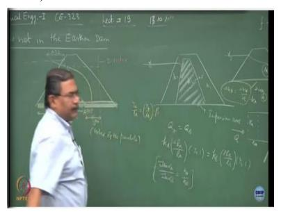
So I may say that y A upon L A is equal to y B upon L B multiplied by some beta, this is my choice. Because this is a geometry, I can control the geometry of the flow or I can assume the distribution of the heads across this point. Ideal situation would be if you keep the head constant between this and this, there is no problem, that is what actually we have done in this case. In the previous lecture, I had stopped after discussing the case of the sheet piles.
