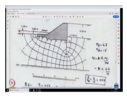
So this is the cross section of the dam which is retaining water with a water head of 5 meter and downstream side you have a water tail of 1 meter. As a thumb rule is that tail water level is considered as datum, draw the flow net number 1, find out the NF ND. So I think now you can realize that drop number 1, 2, 3, 4, 5, 6, 7, 8, 9, 10, 11, 12, 13, 14, 15. So I have drawn ND as 15, the flow lines would be 1, 2, 3, 4 and then some fraction of the squares which I am considering as 0.7.
