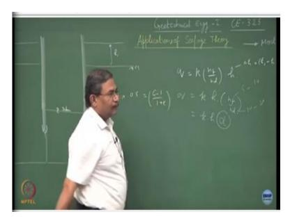
And I think I have introduced this concept that q = k into nf upon nd multiplied by h, where he is nothing but delta h. So, h could be the delta h, h1 - h2, nf is the number of flow channels, nd is the number of drops of the equipotential line. Having done the flow net, start counting, this is the equipotential, this is the bottom most flow line impervious layer. So, no discharge is going to take place through this, good, sheet pile no discharge across this.
