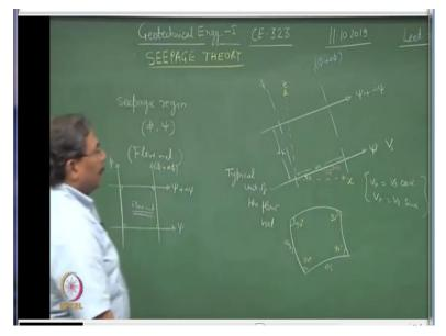
So suppose, if I assume that this is the psi + delta psi and there is another flow line, which is depicted as psi. Now perpendicular to this would be the equipotential functions depicted as pi + del pi. In such a manner that this is delta s distance and this is the delta n. So there is a specific reason of assuming this as delta s and delta n, this is the direction of the flow. So that means, the discharge velocity is in the s direction.
