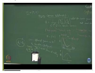
This is wet of optimum you should correct me and this is dry of optimum alright. So dry of optimum we have particles which are highly disoriented alright, we call them as flocculated and on the wet of optimum we have the particles which are more dispersed. So by definition or by fundamental nature a dispersed structure shows less hydraulic conductivity as compared to the flocculated structure then we talk about the formation also.
