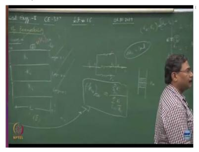
So if I consider is layered system of soil mass, so this is layer number 1, layer number 2, layer number 3 and so on. We might be having layer number n as well alright, I repeat is a inhomogeneous system heterogeneous system of soil mass. Because you have different layers, but what we are assuming is that each layer is isotropic in nature that means at a given point the properties, density, void ratios, hydraulic conductivity are going to be constant.
