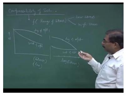
So I was talking about the compressibility here. Normally compressibility is a function of range of stress. Sometimes we define things as a low stress and sometimes we define this as the high stress. So, suppose if I plot void ratio as a function of stress, I will use that term as stress for the time being when we are dealing with the low stresses in ranges of kilopascals fine. This is the response of the soil on the dry of optimum and wet of optimum.
