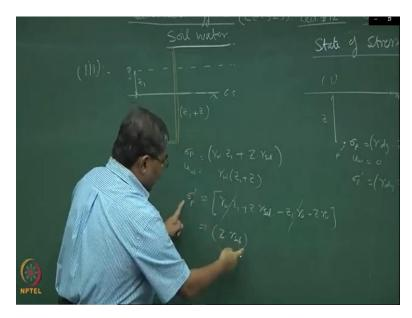
This is the ground surface and during rains, what is going to happen. Suppose if this is the point P water logging, is this correct, says z 1 and this is z, what is an intuitive feeling what has happened to sigma p and you w. Quickly, sorry, yeah, do it systematically. So, sigma p will be equal to gamma w z 1 + z gamma saturated, is this okay. This is the overweight and up to this point this is the whole system water table is here. So, the whole soil mass is saturated.
