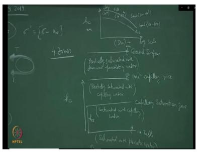
They are normally 4 zones of soils. The ground surfaces is this. There is something known as maximum capillary zone or sometimes it is also write it as maximum capillary raise. Then we have, I should not show it as the water. This is the capillary saturation zone and this is somewhere the water table is. This is what I have defined h c, in some of the books you will find this h c as h c max also.
