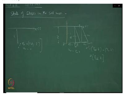
State of stress in the soil mass. Let us start with the simple ground surface and at a depth z, I
