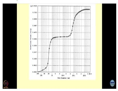
So, let us interpret one of the typical graphs that you will be getting from MIP. So this is an intrusion curve, that means the Mercury is being intruded into the pores. So, as the pressure here I have plotted pore diameter, which is inverse of the pressure. So, these are the coarser pores, and these are the finer pores. And this is the normalized volume that means the volume of the Mercury which enters divided by the volume of the sample.
