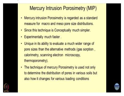
Rather than discussing this, okay let me give you a quick idea about what MIP is so, this is a standard method for determination of macro and mesopore size distributions. And it is a very simple technique where you are intruding Mercury into the sample under some pressure so conceptually do the simple thing. Mathematical modelling is quite easy, easy to conduct the experiments.
