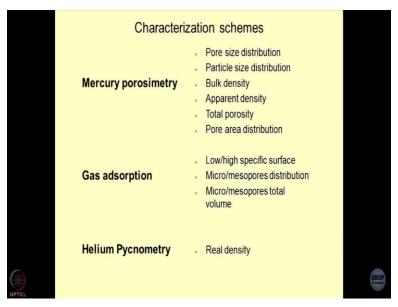
These are the guidelines which are normally used, which equipment should be used for what type of characterization of the geomaterials, so we have three techniques. That is the mercury porosimetry, gas absorption and the helium pycnometry. And these instruments are becoming very common in the environmental geomechanics laboratory. Helium pycnometry gives you the real density. Real density, the specific gravity which is skeletal.
