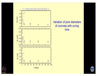
So, this is a good example of how it varies over a period of time in case of concrete which is getting cured. Why I am citing this example is concrete is still a very stable material as compared to the soils. But when I deal with the minerals which are active or the processes which are very active as a function of time inside the soil matrix, it becomes very difficult to capture the phenomena by using MIP.
