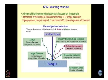
This is the working principle of SEM, a beam of high electric, high energy electric electrons is focused on the sample, and then the interaction of electrons is transformed into a threedimensional image to obtain the topography, morphology and composition and crystallography of the grains. So, topography, morphology and compositional characteristics I have discussed and crystallography is basically how the crystal structure is changing.
