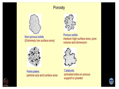
And another interesting thing is, I hope you should realize that porosity is something which could be in any of these forms. This is a non-porous solid for that matter a perfect quartz grain of the sand. Now, this has an extremely low surface area because there is no cation exchange capacity, it is quartz is a very dull material, it has no affinity towards the external environment All right. So, truly speaking non-porous solids are made up of quartz. Quarzitic material.
