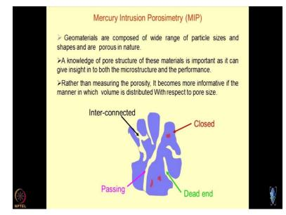
So, porosimetry is becoming very, important in the realm of environmental geomechanics because of the obvious reasons that pores are the ones which play an important role in any mechanism which occurs in the geomaterials. Transport of mass flux alike. So, this flux could be thermal, electrical, chemical, biological, radiological, magnetic, and so on. So, until now, we have been talking about only the particle size distribution in conventional geomechanics.
