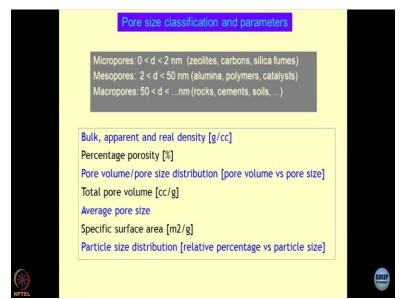
When we talk about the pore size the in geomaterials, we use this classification scheme, Micro Meso and macropores. So, as the name suggests, the micropores are going to be the smallest ones, then we have in between, and the macropores are the big pores. So, up to the 50 nanometers and more than that, these are the micropores, and the smallest pores are less than 2 nanometers. So, most of zeolites carbon silica fumes which you have studied would fall under the category of micropores.
