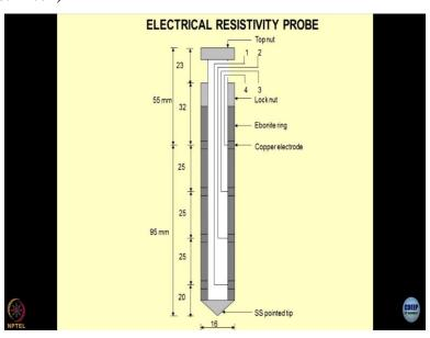
My student Reshma created this probe which is now Dr Reshma. This is an electrical resistivity probe, very interesting way of measuring the electrical properties of the geomaterials in their compacted form, what we have done is we have taken a cylindrical rod, and on this cylindrical rod, we have placed four electrodes. So, this is one ring electrode, another ring electrode and another ring electrode.
