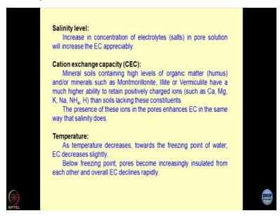
It is all about the conduction of the electrons or the current. Salinity level. So, when the more
