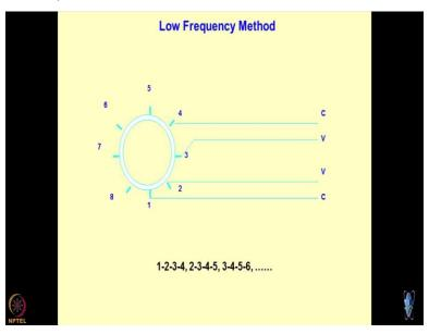
Based on this, some people have done a consolidation test by inserting electrodes into the odometer cell. And what they have done is they have placed let us say eight electrodes. These are point electrodes, small pins which have been inserted into the sample holders or the odometer cells of certain diameter made up of stainless steel. So, this becomes an electrode and what they have done is they have measured the properties of the soil across four-electrode.
