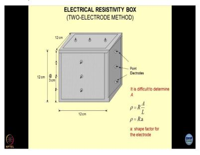
We went ahead with another type of box where we embedded three electrodes on each face of the box. And then we measured the electrical properties across the pair of electrodes. I hope you can realize that the efforts were on to find out the equivalent circuits for the geomaterials because this point electrode and the one who is hiding behind would form a pair of electrodes. So, across the vertical plane, I can get three values of the resistance and the capacitance and inductance.
