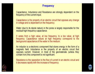
A little bit on the frequency of the current because this governs the whole process and the mechanism. Though I have talked about the low-frequency domain and the high-frequency domain, I am sure in your 10+2 physics you must have studied that how the capacitance, inductance and the resistance depending upon the frequency of the current is it not. So, this concept can be utilized to see whether material is conducting or an insulator.
