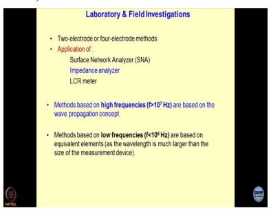
I will come to the laboratory and field investigations. Simple experiments can be done in the laboratory by adopting two electrodes configuration of 4 electrodes. And the applications are sometimes we use surface network analyzer Also, if you have done a course in electronics in your undergraduate, you must have used this SNAs, surface network analyzers, if you want to find the fault in a cable system or where there is a short circuit which has occurred.
