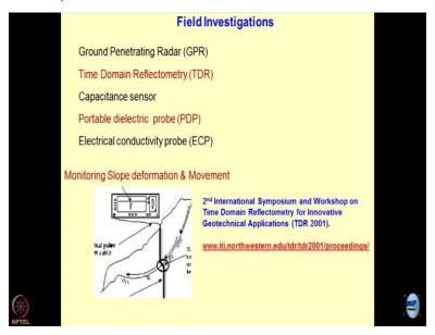
Some field investigations which are becoming very popular in these days, where the GPR is the leading example, from ground-penetrating radars, TDRs are being used for finding out the subsurface profiles of the material and the capacitance sensors which are used for finding out the degree of contamination of the geomaterials. There are portable electric probes also which are available in the market.
