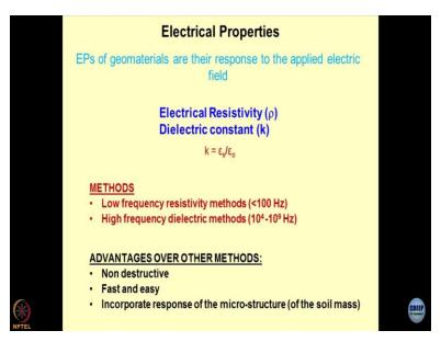
So the electrical properties are electrical resistivity in 10 + 2 physics I am sure all of you have started and the dielectric constant K. So, there are two broad methods of determination of electrical properties. One is we call as low-frequency resistivity methods where the frequency of the current is less than a hundred hertz. However, there is a second category which is known as high frequency, electric methods, where the frequencies are up to the order of mega to gigahertz.
