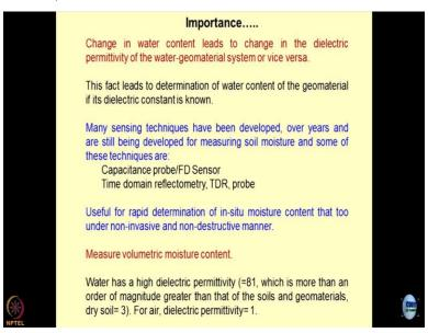
Another set of importance is that these are the concepts which have been used in understanding the electrical properties of the geomaterials. The basic hypothesis is that for any material, the dielectric constant of the dielectric permittivity defines its properties. In other words, for every material, there will be a unique dielectric constant. And the reason is that most of the geomaterials are made up of oxides of silica element ion, sodium, potassium, calcium and so on.
