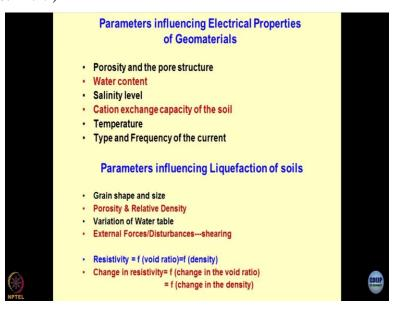
Now, comes the parameters which are influencing the electrical properties of geomaterials, porosity and the pore structure is number one. And because the passage of current through the geomaterial is because of its inherent porosity and its pore structure, so I am sure you have come across these concepts of why permeability is more in the flocculated state of the geomaterial or the soils as compared their dispersed state.
