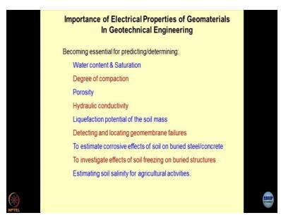
So, to begin with, what are the importance of electrical properties of materials in contemporary geotechnical engineering, this becoming essential for predicting and determining the most fundamental parameter related to the geomaterial which is the water content and saturation. See gone are the days when people used to take out samples from the field, and they used to test them and then they used to analyze the results.
