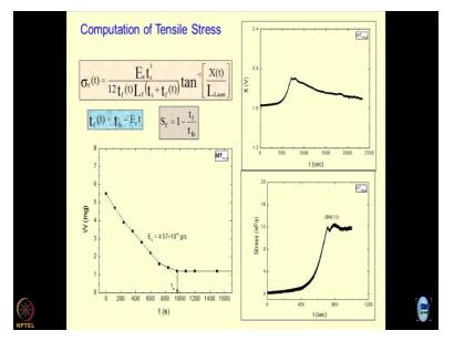
And I can obtain the  $\sigma_t$  as this function. So, x upon L is nothing but theta term, and I can find out what is the final thickness of the clay film if the initial is known and Er is the evaporation rate multiplied by the time. So, if you take the sample in the petri dish and expose it to the environment as the weight loss occurs after a certain time the weight of the petri dish becomes constant, this is a critical time the slope of this line is going to give me the elastic modulus.
