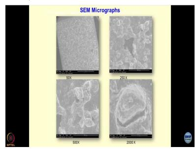
And we did the complete SEM micrographs of the process to understand how the cracking gets initiated in the clays, this is the initial sample and hope you can realize that there is an opening up of a crack at different magnification this is how the crack initiation occurs. And if you see it at very high magnification, this is how the cap gets opened up this cracks develop in the whole system we wanted to make a video of the entire process. It requires very expensive setups for that.
