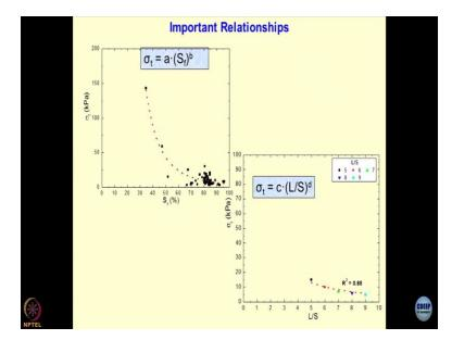
And from these simple experiments, we did some relationships where the tensile strength has been linked with the thickness of the film of the clay. And tensile strength has been with the L/S ratio that is the liquid to solid ratio of the clays. These are the topics of multi-phase geomechanics, those of you who might be interested or might land up doing this type of R and D would be dealing with these type of problems, which are very intricate, very very complicated and they test your nerves.
