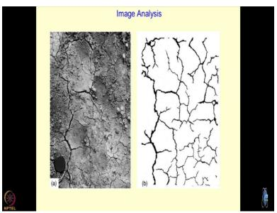
This is what happens in nature. This was a project, which I was doing for a huge reclamation, which was going on in one of the ports. And the question is, if you are not using the right type of the soil, even after the pad is constructed, the entire thing will crack, and your filling will become
