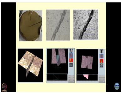
If I start with the sample, you can see very clearly the cracks growing in different directions; I wanted to study the depth of the crack which gets developed. This is how the greyscale model
