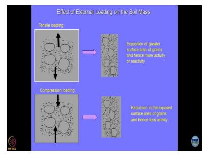
So, if you start with, let us say tensile loading or the compressive loading, and these are the grains, which are in the soil mass, and if I stretch it, what is going to happen, when I stretch it, all the particles get repelled from each other. That means, in other words, each particle is now free to exhibit the 100% surface area to the environment. So, this is a case when tensile loading causes, exposure of the grains to the environment.
