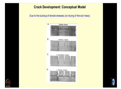
Now, if you think about the conceptual model that why soils crack, the tensile stresses which develop in the system to be blamed for cracking of the soils and tensile stresses develop due to the desiccation of the soil mass or the drying of the soil mass. So, I am sure you must be realizing that this is a situation which does not occur because of the mechanical loading of the soils.
