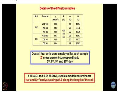
So, we did several tests by taking the soils of different types with different saturations. 100, 80, 60 corresponds to saturation levels, the moisture content and the volumetric moisture content and different densities. These are two different types of soils. And what we have measured is that we have measured the impedance. So, I will show you quickly how this impedance can be of some help in establishing the migration of diffusive contaminant front.
