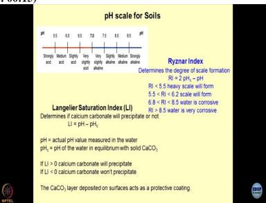
So, the LI of the Langelier Index this is defined as the pH of the water actually, then pHs is the pH of the water in equilibrium with solid calcium carbonate. Now, this shows how much unsaturated the water is in terms of calcium Ions. Now I hope you can understand if LI is greater than 0, that means pH is of the water is more than the pH of the water when it is in equilibration with calcium carbonate.
