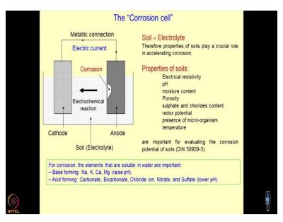
So, this is the conceptual discussion on corrosion cell. Now, what it indicates is that if I take the soil mass, which is not dry. So, maybe during rains, the soils will become wet. And once the sides become wet, the electrolyte gets developed over there. This could be because of the groundwater. Also, the moment soil becomes wet, there could be a situation where cathode anode might get developed, do not think that cathode has been inserted into the soil mass.
