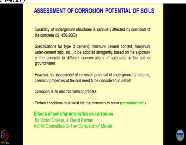
Now, whatever we did, I am just going to present the assessment of corrosion potential of size. So, when we talk about the underground structures and their durability, there is a code IS code 456 you must also studied 2000 on the corrosion of concrete. What are the types of cement should be utilized? There was a time, and some of the cement industries used to contact me for doing micro zonation of the soils, where most of the infrastructure is going to come up.
