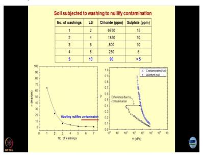
And we started washing them to nullify the contamination level. So what we will observe here is that we have given number of washings to the soil sample, LS is the liquid to solid ratio, process simple, you take a certain amount of soil and add two times the water. So, this becomes L/S is equal two measure the chloride content and sulphite content and keep on increasing the volume of the water to wash the soil sample, or you can literally wash it also.
