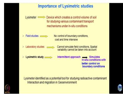
What is the importance of the lysimetric studies this was a project which I did for Atomic Energy Regulatory Board of India and BARC. So, as I said, the lysimeters are basically the devices which create a control volume of soil for studying various contaminant transport mechanisms under in-site conditions. There are 2 types of this field and laboratory studies in field studies unfortunately not much control on the boundary conditions and they are very expensive and very time-consuming.
