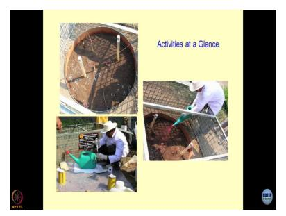
Just to show you how the activities are done in the field. This is how the whole system has been created the two SS tubes are fitted for suction samplers are fitted; these are the cubes which are connected to the suction samplers. Now, you can see that we are giving, this is the strontium crimson red colour is the typical colour of the strontium radionuclide and then we leave this whole thing for rainfalls to come.
