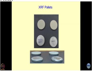
So, just to give you an idea about these are the XRF pallets if you get a chance go to the SAIF and you can see how these pallets are done. These are small aluminium pallets, half of them is filled with the adhesive these all standard methods nowadays they will help you. So, half of this is filled up in cellulose, and the rest of the half is filled up with the material for which you are trying to find out the chemical composition.
