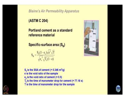
This is a Blaine's Air Permeability Apparatus you must have used it; this is a U tube, and in the U tube one part of the U tube is connected to pump air pump like the blood pressure machine, and this is a sample holder. So, in a hole weight of the sample is compacted in the sample holder, and this is attached to Blaine's air permeability apparatus. And what you see over here is the mercury column.
