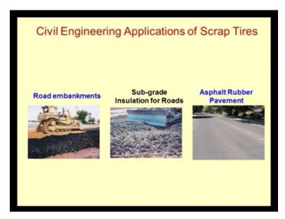
There are several applications on the scrap tires, and some of them are road embankment. You can shred the tires, you can use them as aggregate for making the road embankments, and I am sure you will realize that once the shredded tires are being used the elastic modulus and the bouncing property of the finished surface are going to be much better, and damage to the automobile vehicles tires would be extremely less as compared to the rigid pavements, which are fairly aggressive.
