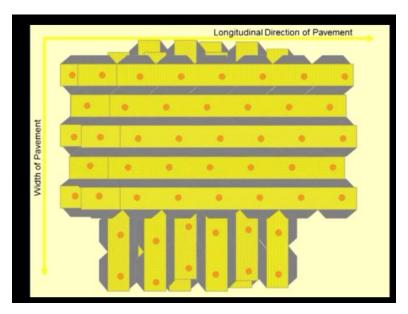
So, if you talk about the width of the pavement and the longitudinal direction of the pavement, you can stack these units one by one, and you can rivet them by using anchors. The next layer would come off another layer of anchors followed by another layer of the sliced rubber tires and keep on repeating this as long as you achieve the desired height of the system. So, I am sure you must be realizing. This is a good, clever idea of utilizing industrial byproducts.
