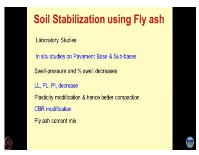
I am sure you must have come across different types of application of the fly ash. So normally people have used the fly ash for stabilization of roads increasing their CBR pavement and subbases their properties. People have used fly ash for reducing the swell pressure of the soils so by addition of the ash into clays and particularly the clays are swelling type you are neutralizing the swelling effect as well as very high liquid limit and plasticity index.
