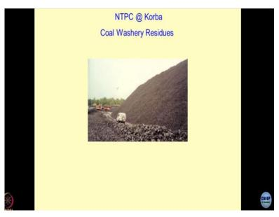
I hope you can realize now the magnitude of the problem. Had it been some embankment I would not have bothered much about it, but this is carbon material is it not. The chances of this metal catching fire during summers are tremendous. Methane formation is taking place because of coal, so flashpoint is their organic material, and you are stacking it like this. It is a hazard to store this material in your premises clear.
